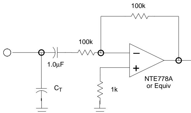
$C_T = 20\text{pF}$  = total parasitic capacitance, which includes probe, wiring, and load capacitance
