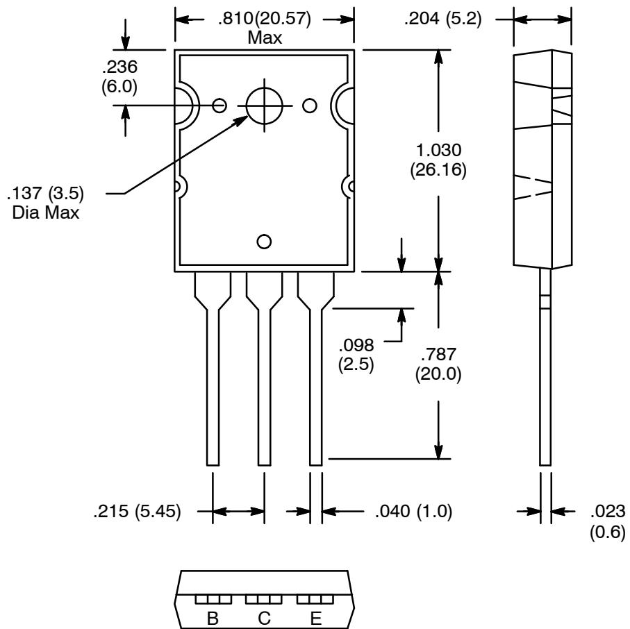
**Note:** Collector connected to heat sink.
